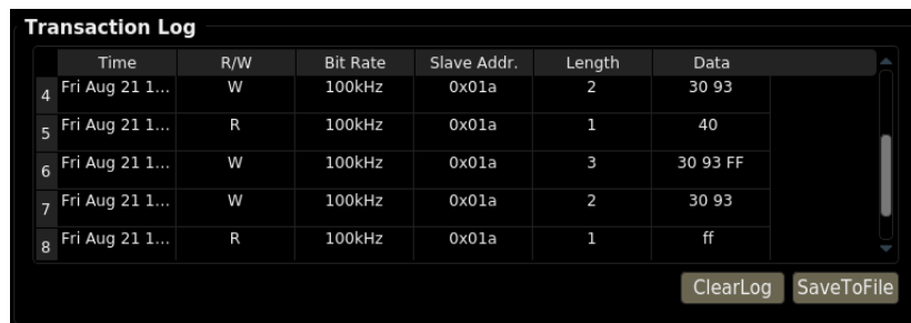
Figure 6.25. I 2 C Master Register Read
