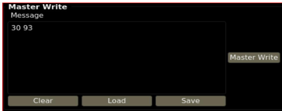
Figure 6.19. I 2 C Master Write to Write the Register Address
