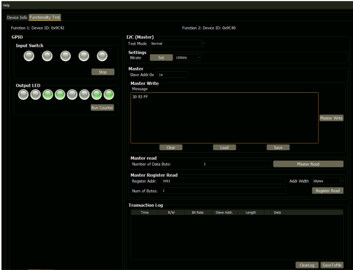
Figure 6.5. Functionality Test Tab for CertusPro-NX
