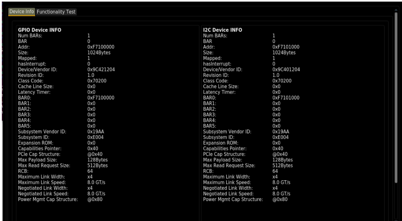
Figure 6.2. PCIe Test Application Device Info Tab for CertusPro-NX
