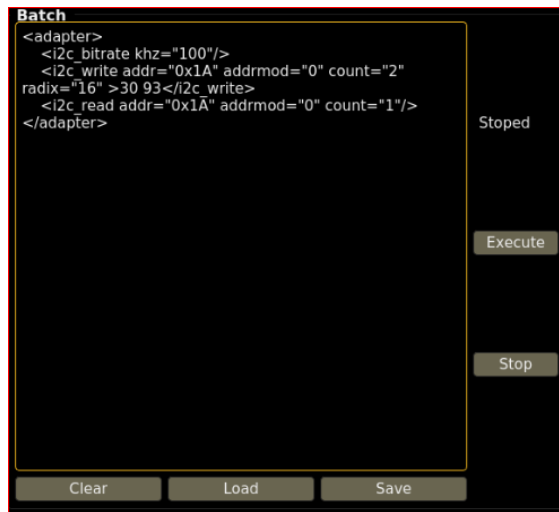
Figure 6.25. I 2 C Batch Mode Read/Write
