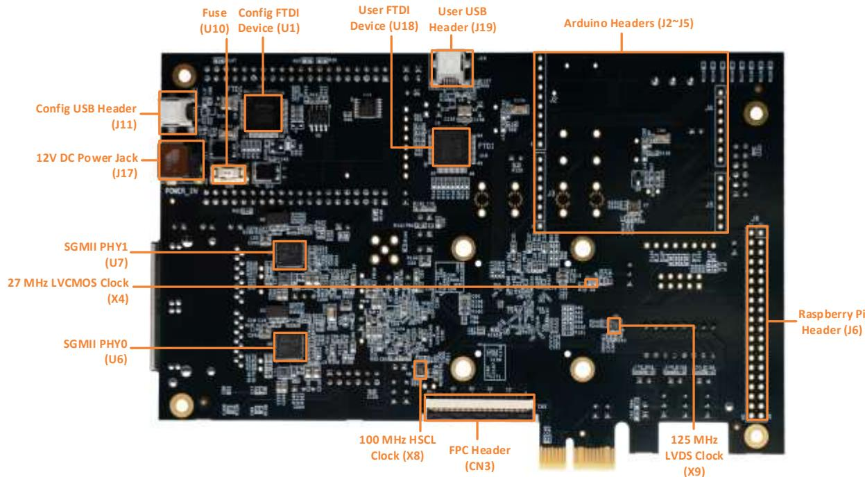
Figure 1.2. Bottom View of MachXO5T-NX Development Board
