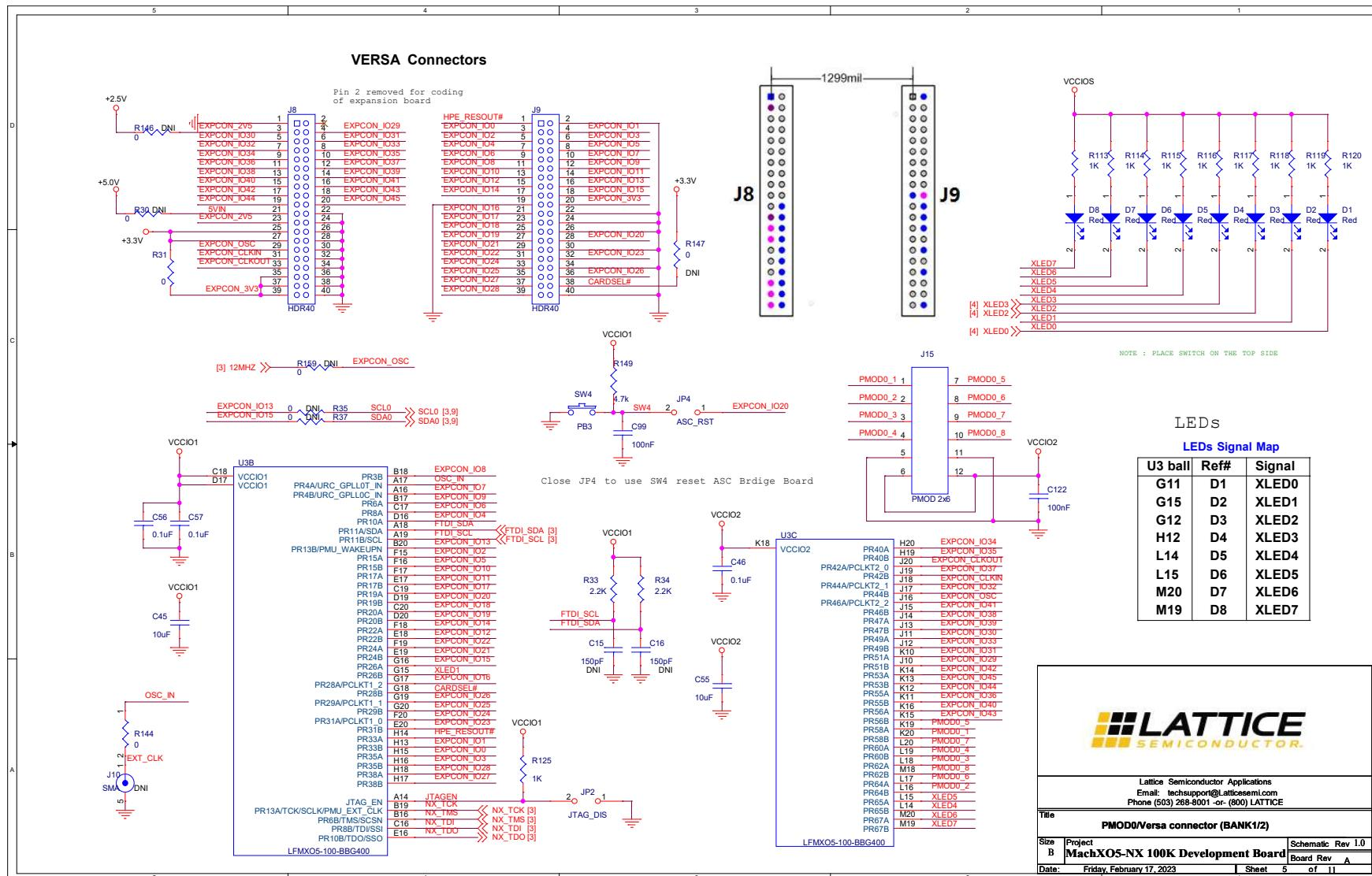
Figure A.5. PMOD0/Versa Connector (BANK1/2)
