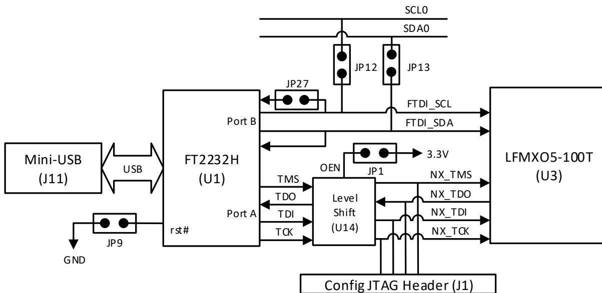
**Figure 3.1. JTAG/I<sup>2</sup>C Programming Architecture**
