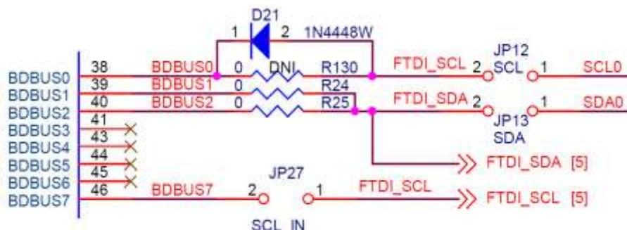
**Figure 3.5. I<sup>2</sup>C Programming Mode**
