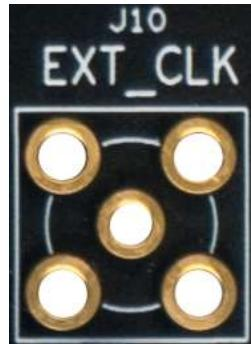
**Figure 8.3. SMA Clock Input**
