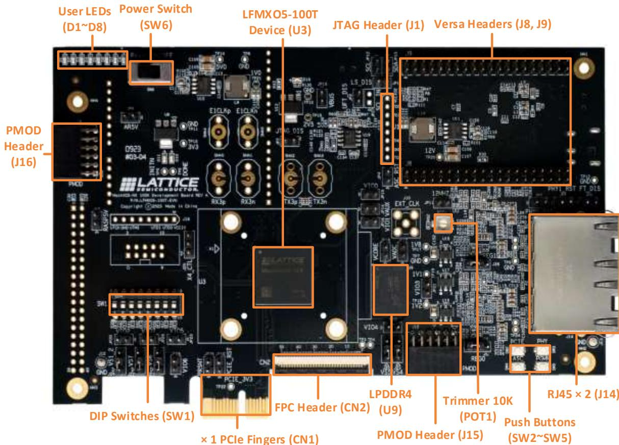
[Figure 1.1. Top View of MachXO5T-NX Development Board](#)
