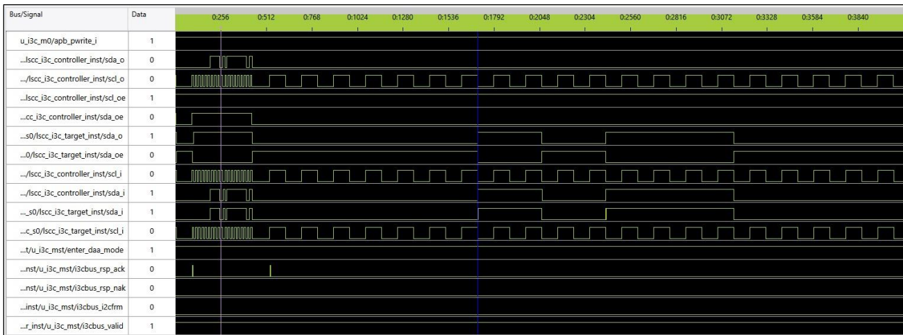
Figure 6.9. Sample ENTDA sequence sent by I3C Controller
