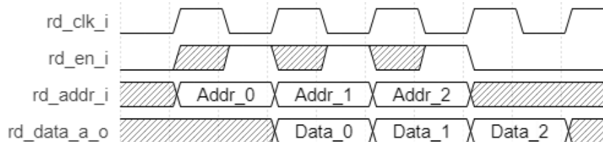
Figure 2.9. Distributed Read Only Memory Timing Diagram, With Output Registers
