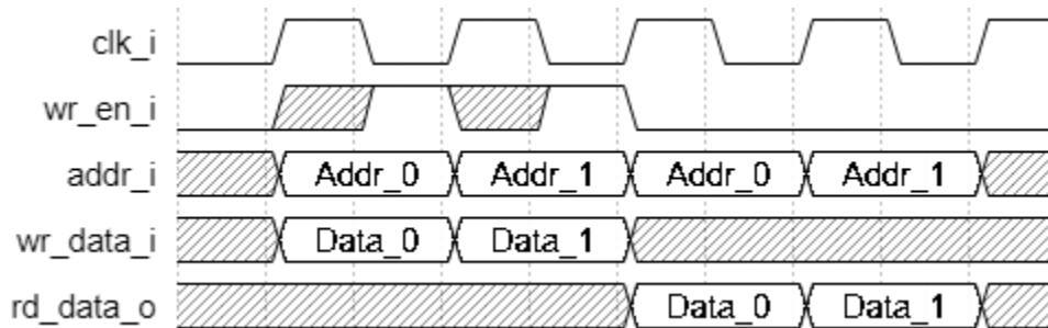
Figure 2.2. Distributed Single Port Memory Timing Waveform, Without Output Registers
