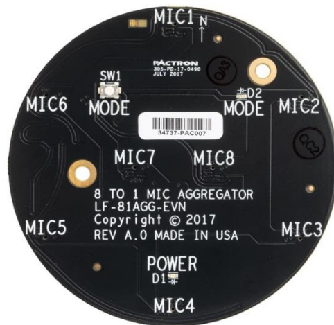
Figure 3.2. 8 to 1 Mic Aggregator Board (Daughter Board)
