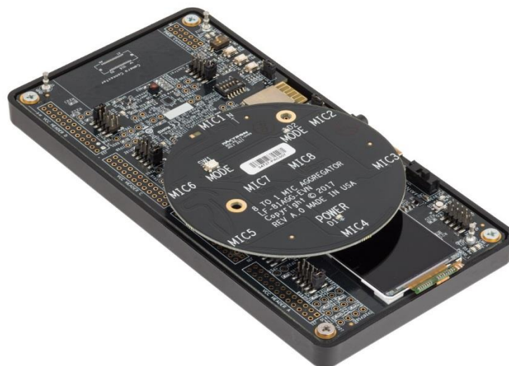
Figure 3.3. iCE40 UltraPlus MDP and 8 to 1 Mic Aggregator Board
