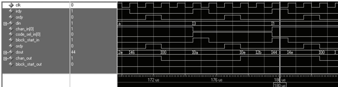
Figure 4. User Interface Timing Diagram for Two-channel Correlator
