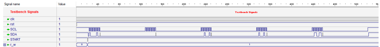
Figure 9.7. Simulation Waveform Showing a Four-Byte I 2 C Write Transaction with Clock Stretching
