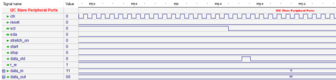
Figure 6.4. Zoomed-In View When 0x11 is Fetched by the I 2 C Slave Module
