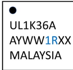
**Figure 1 – Date Code Identifier for ASEM**
