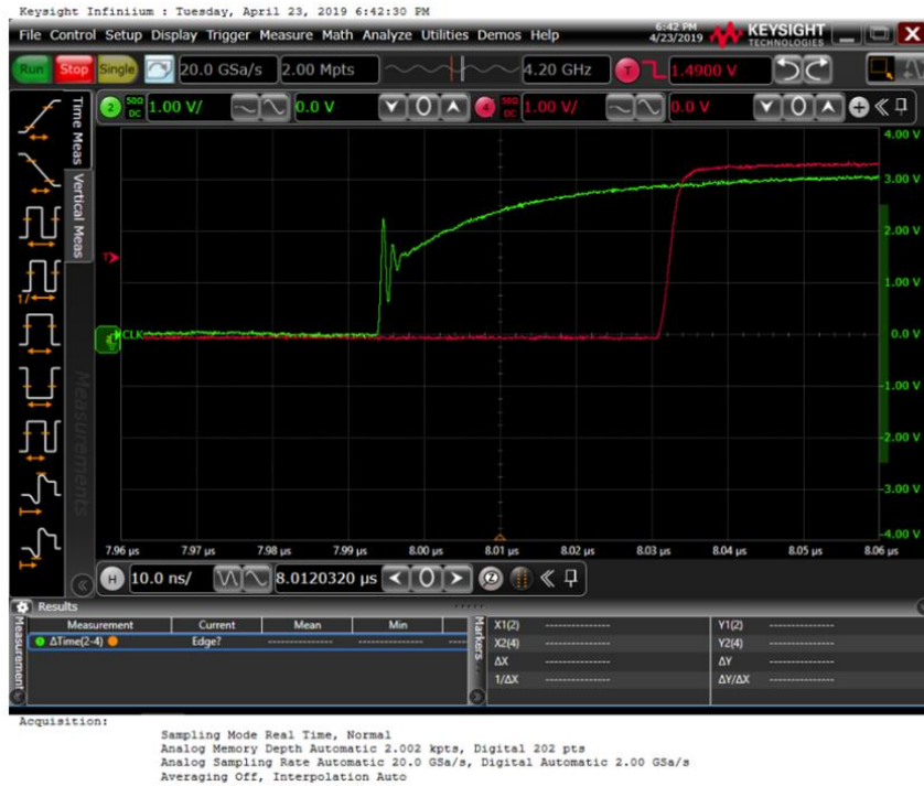
Figure 2. Issue #2 – Race Condition between OE and Logic Level can result in ringing.
