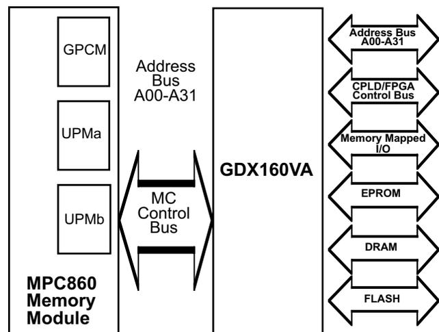
Figure 2. CPM/GDX160VA Block Diagram
