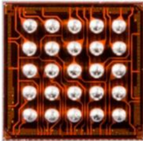
Figure 1.1. 25-Ball WLCSP Package (Actual Size: 2.5x2.5 mm)
