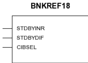
Figure 2.2. Primitive for Bank Controller
