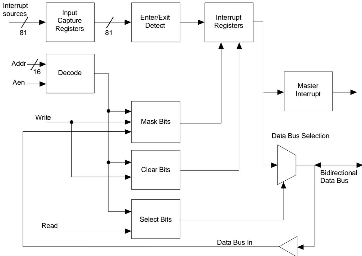
microprocessor and the input of the bi-directional data bus are used to generate the mask bits and to clear bits for the interrupt registers.
