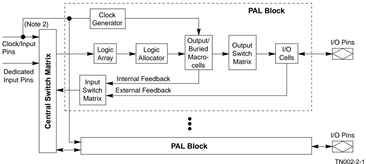
**Figure 1. MACH 4 Block Diagram and PAL Block Structure**
