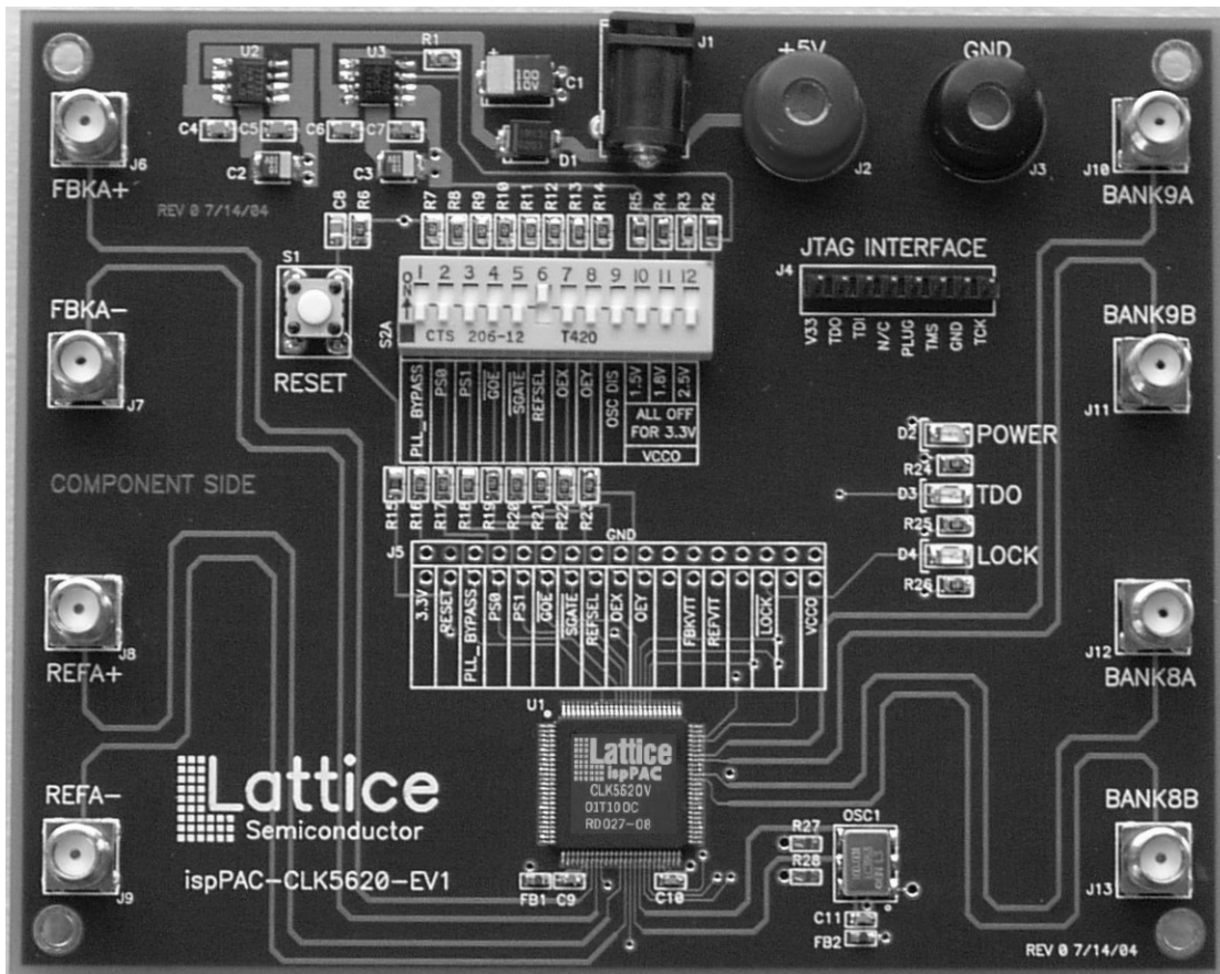
Figure 1. ispPAC-CLK5620-EV1 Evaluation Board
