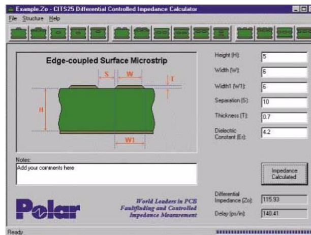
Figure 5.5. Differential Microstrip Example with Polar CITS25 Impedance Calculator Tool
