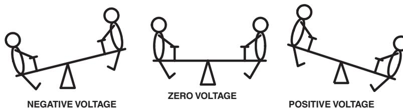
Electrically, the two seesawyers are replaced by a pair of wires labeled  $V_+$  and  $V_-$ . When  $V_+ > V_-$ , the signal is defined as positive, while when  $V_+ < V_-$ , the signal is defined to be negative.
