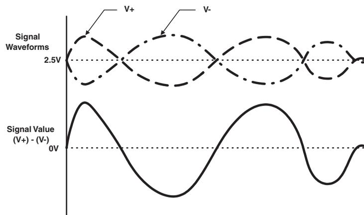
The average voltage around which the differential pair of Figure 2 swings is set to 2.5V and is after referred to as the 'common-mode' component of the differential signal. Offsetting the pair in this way provides the maximum range of signal swing when the individual members of the pair are limited to a 0-5V excursion. This is often the case when operating from a single 5V power supply.
