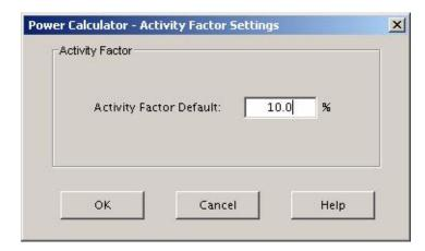
All the default activity factors appearing in blue font on the Power View and Icc View tabs are changed to the new activity factor. The Power Calculator automatically saves the new default.
