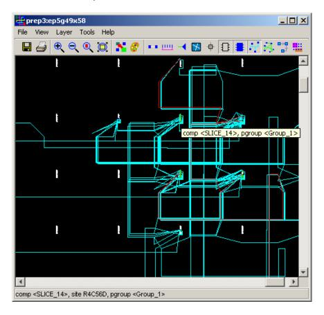
**Path Tracer** The Path Tracer now includes a Grouping button, allowing you to create a physical group from components in selected paths. It also includes a highlighting feature that color-codes selected paths as they are cross-located in the Floorplan View.
