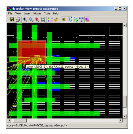
**Physical View** The Physical View provides a more detailed small-component layout of your design and enables you to view components such as switch boxes and pin wires.
