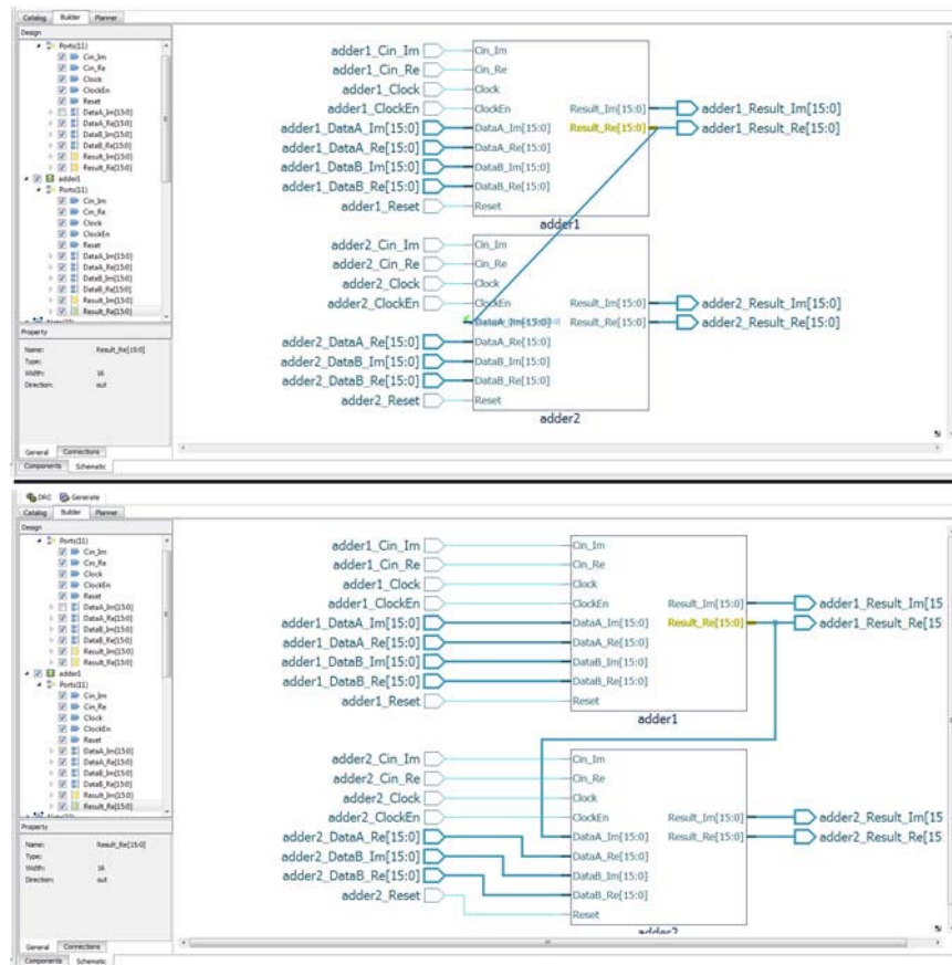
Figure 28: Drag and Drop Connections in Schematic Editor
