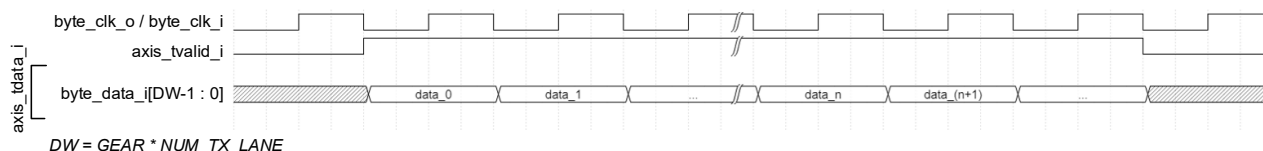
Figure 2.7. AXI4-Stream Enabled and Packet Formatter Disabled Data Format
