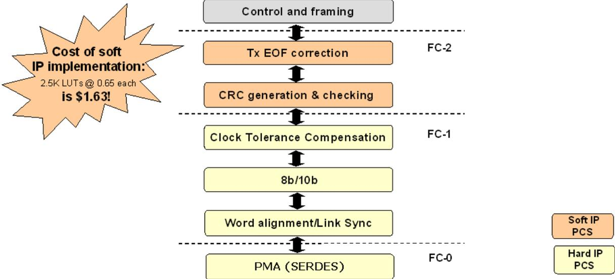
Figure 7- LatticeECP2M Fibre Channel stack implementation
