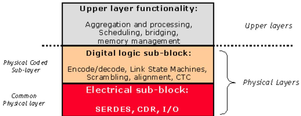
**Figure 1 – Serial Protocol stack functional partitioning**
