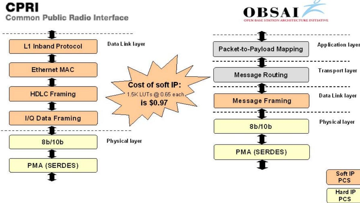
Figure 9 – LatticeECP2M CPRI/ OBSAI RP3-01 protocol stack implementation
