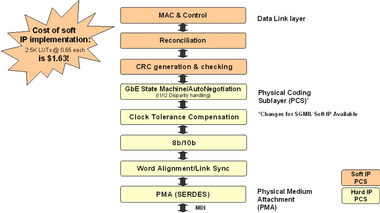
**Figure 5 – LatticeECP2M GbE stack implementation**
