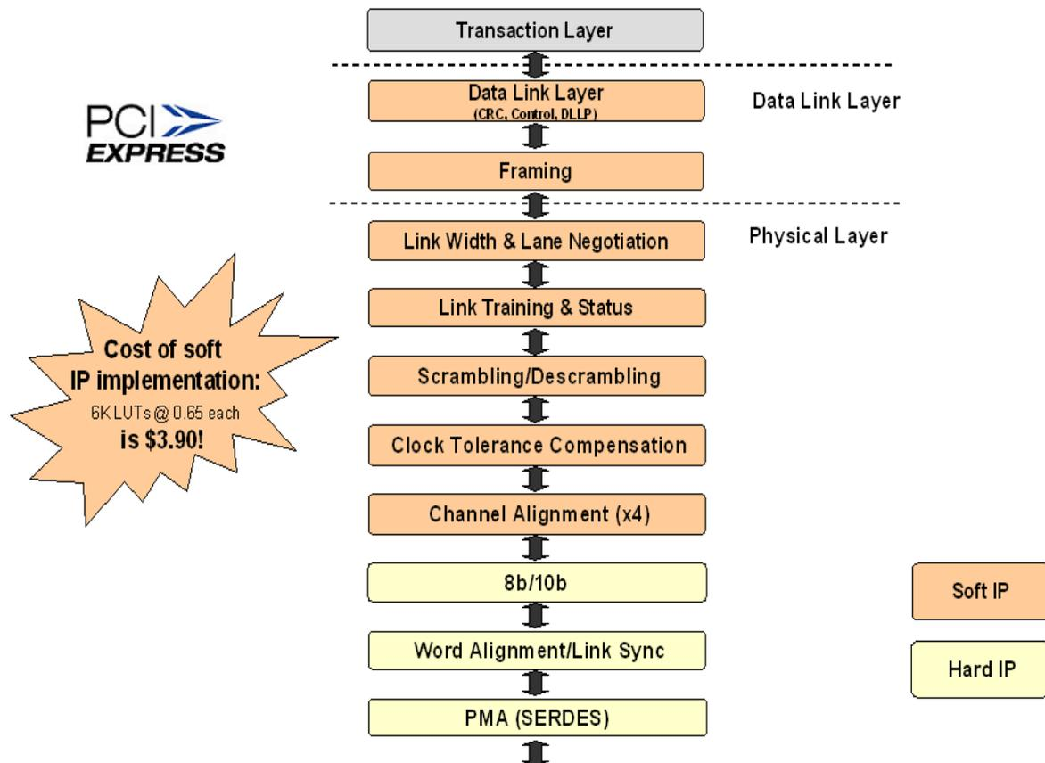
**Figure 3 – Lattice ECP2M PCI Express protocol stack implementation**
