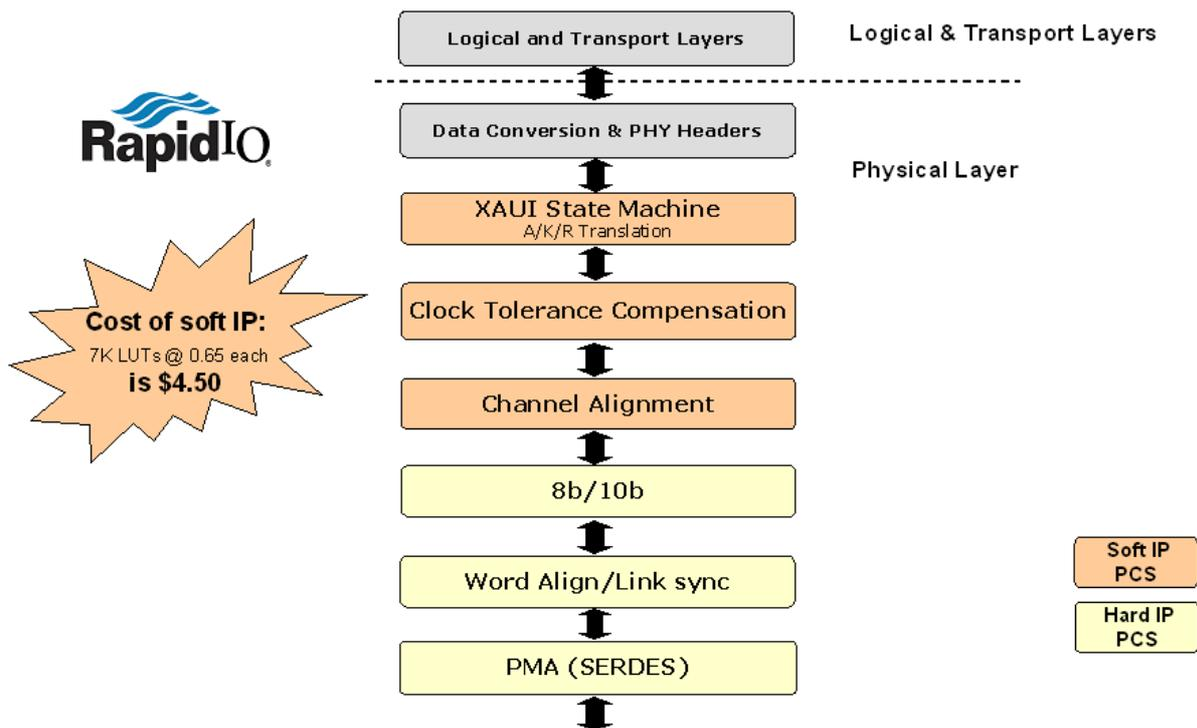
**Figure 4 – Serial RapidIO protocol stack implementation**
