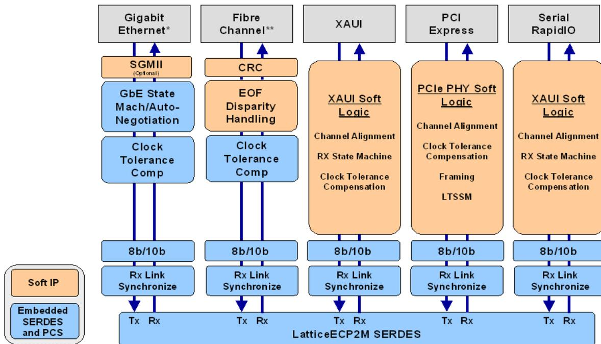
Figure 2 – ECP2M Supported Packet Protocols
