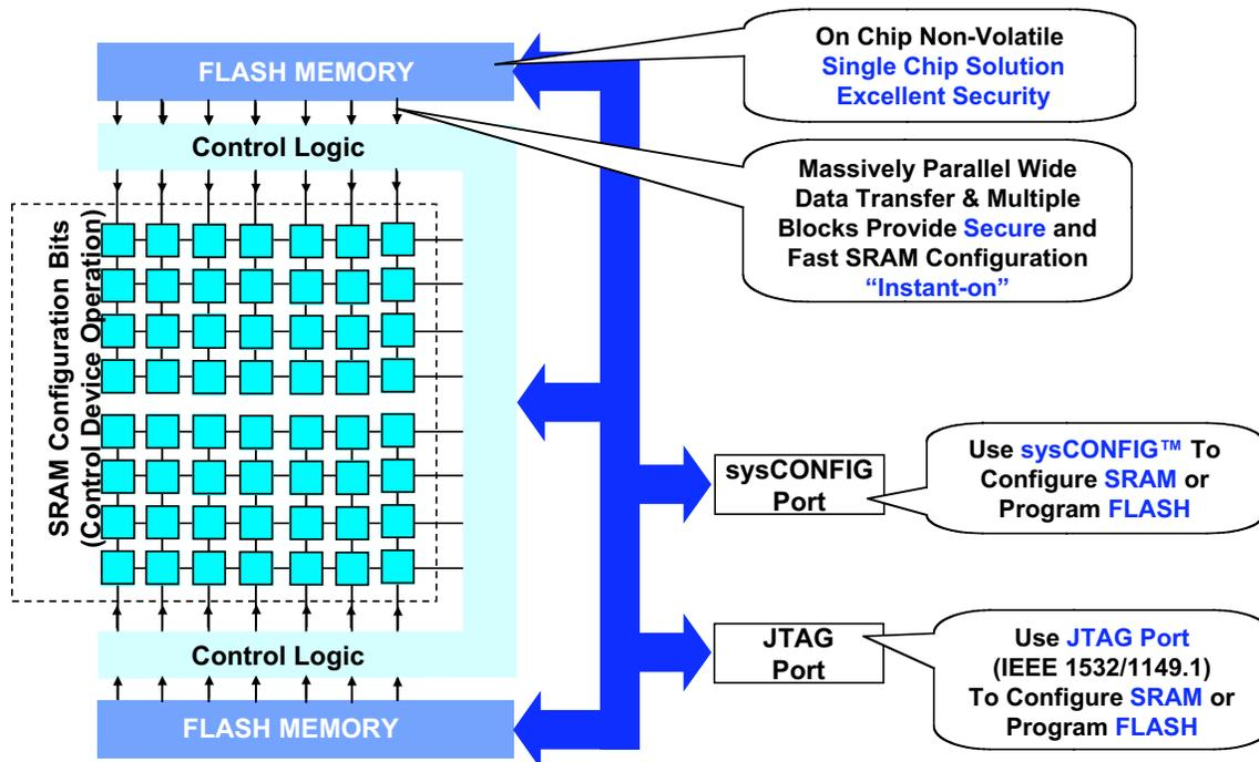
**Figure 6 – Configuration Memories in the LatticeXP**
