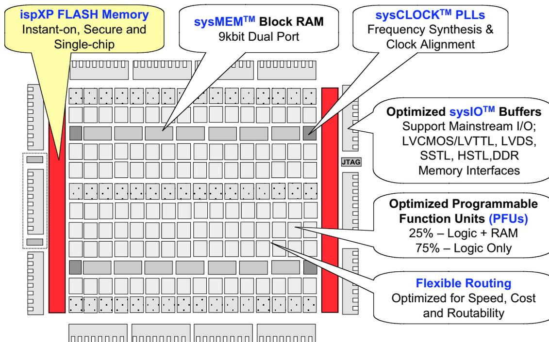
**Figure 5 – LatticeXP Architecture**
