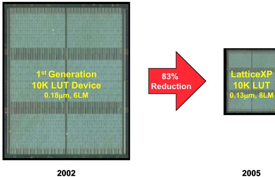
**Figure 2 – 2<sup>nd</sup> Generation Lattice Non-Volatile FPGAs Die Size Reduction**
