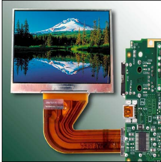
Figure 1 – 7:1 LVDS Cabling for Connecting LCD Screen to Laptop Motherboard
