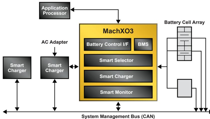
**Figure 5: MachXO3-based battery management system.**
