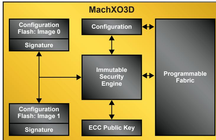
**Figure 4: The MachXO3D's dual-boot capability fully addresses the requirements of NIST SP 800 193 for platform firmware resiliency.**
