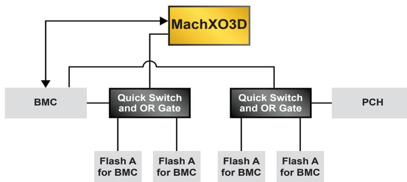
**Figure 6: MachXO3D-based chain/root of trust.**
