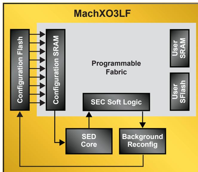
**Figure 2: Simplified block diagram of the MachXO3LF illustrating the soft error detection and correction process.**
