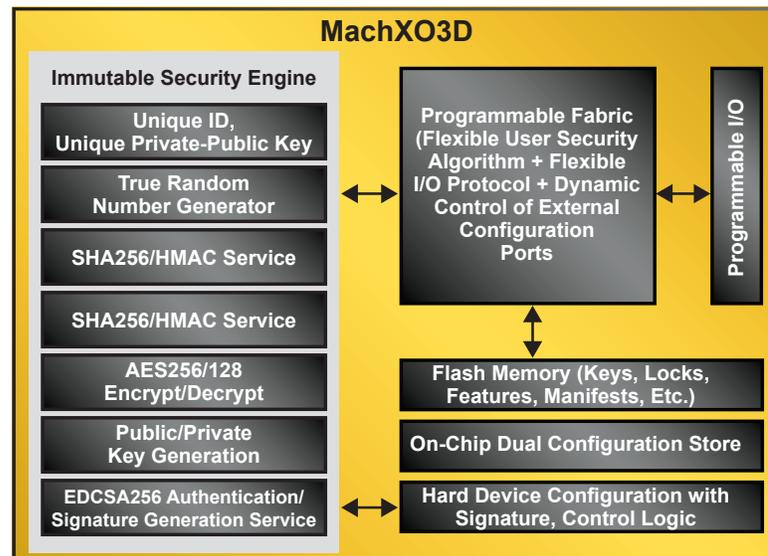
**Figure 3: The MachXO3D secure control FPGA is the system's first-on, last-off, root-of-trust programmable logic device.**
