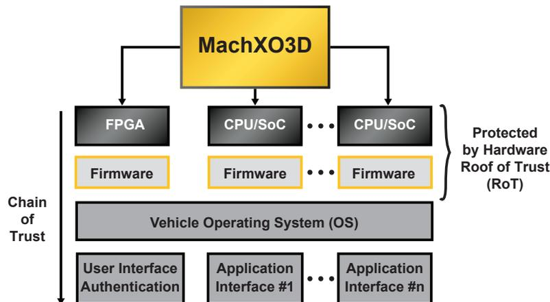
**Figure 7: MachXO3D-based secure boot.**
