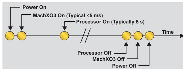
**Figure 1: Dominating the platform control arena, MachXO3 FPGAs are the system's first-on, last-off devices.**
