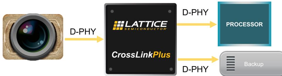
**Figure 5:** In this ADAS vision system, the CrossLinkPlus FPGA is duplicating the camera signal output to send to both the application processor and a data backup.
