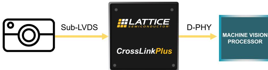
**Figure 3:** In this application example, the Lattice CrossLinkPlus FPGA serves as a bridge between a Sub-LVDS camera and the MIPI I/O on the device's machine vision processor.
