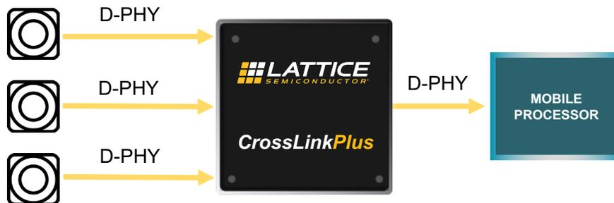
**Figure 4:** Lattice CrossLinkPlus can aggregate multiple sensor signals over one port to conserve processor I/Os.
