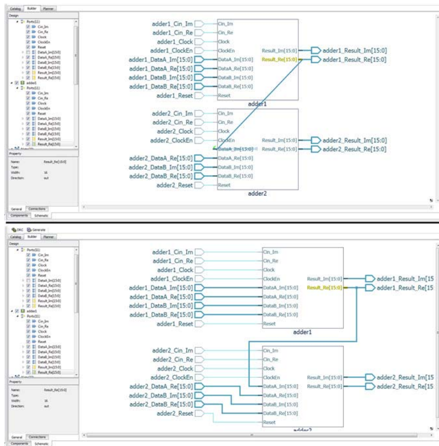
Figure 6: Drag and Drop Connections in Schematic Editor
