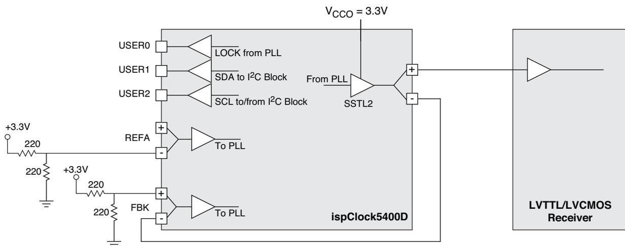
Conceptually, the SSTL and LVCMOS drivers are equivalent since both consist of a pull-up PMOS and pull-down NMOS. The difference in the driver behavior is determined by the off-chip termination circuitry. The LVTTL/LVCMOS input and output specifications are defined in JESD8C, the JEDEC standard for Nominal 3.0V/3.3V Supply
