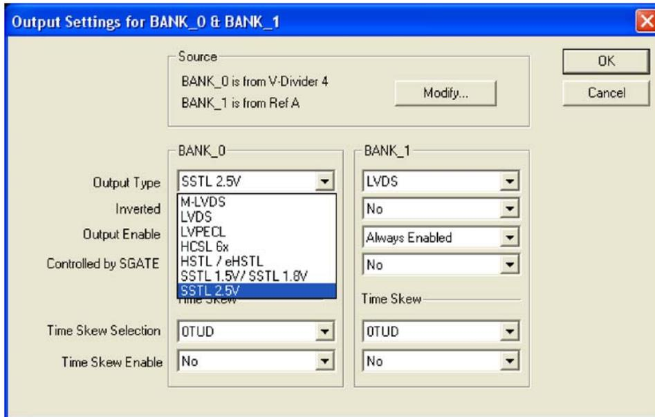
The external PLL feedback is used here to generate zero-delay clock output. Users can make use of the phase and time delay adjustment in the device to further compensate for the board routing delay. The phase skew adjustment can be modified in the Phase Skew Manager block in PAC-Designer. The time skew can be modified in the output block as shown in Figure 2.
