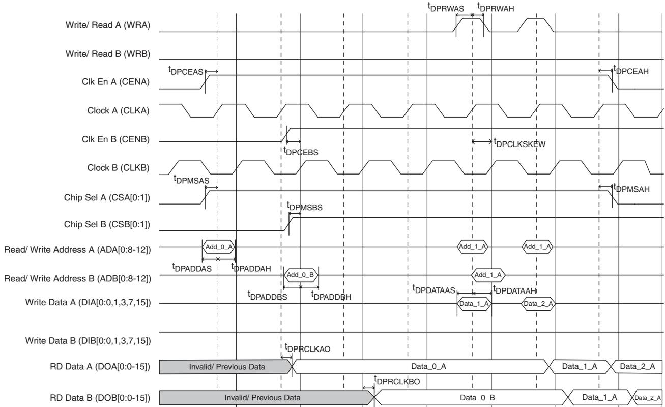
Note: While one port is writing and the other port tries to read or write at the same memory location, there must be a minimum  $t_{DPCLSKKEW}$  between the two clocks.
