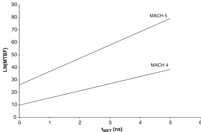
To calculate the stabilization time based on the MTBF:
