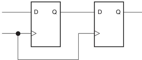
Note that each extra stage of flip-flop means an extra clock delay for the data must be absorbed by the system. This method is not foolproof. The possibility of metastability is reduced, but not eliminated. A flip-flop can go metastable if the preceding stage does not recover quickly enough.
