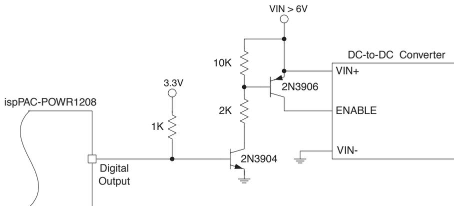
In this circuit, the collector of the NPN transistor now stands-off the VIN+ voltage instead of the ispPAC-POWR1208's output, offering compatibility with higher VIN+ voltages, depending on the choice of transistors. The addition of the extra transistor also has the effect of inverting the ispPAC-POWR1208's digital output, so that the PNP transistor is now turned ON when the digital output is HIGH. Note that a similar solution using opto-couplers will be discussed later in this application note.
