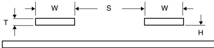
**Figure 5. Edge Coupled Stripline (Sandwiched Between Two Reference Planes)**
