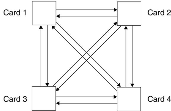
Each card must provide 3 transmitter and 3 receiver ports. Each arrowed line represents a point-to-point backplane net.
