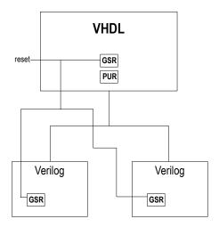
A GSR component should be instantiated in the VHDL top hierarchy and connected to the desired reset signal. A GSR component should be instantiated in the Verilog hierarchy and connected to the same reset signal. If there are separate Verilog hierarchies within the VHDL top hierarchy, each Verilog hierarchy must have its own GSR component instantiated and connected to the reset signal. GSR components instantiated in one Verilog hierarchy do not affect other Verilog hierarchies.
